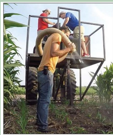
HAIL MACHINE: Justin McMechan pelts young corn with the hail machine as part of his research to more accurately assess initial hail damage and the corn plant's ability to recover.
